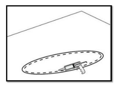
Step 5 Apply a thick bead of silicone within bath outline. Use the appropriate silicone for the surface type.
