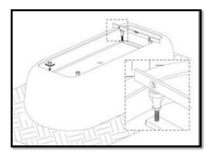
**Step 1** Ensure legs are adjusted in line with the base of bath. Assemble The bath on a mat to ensure against any damage.
