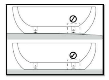
**Step 2** Check that the bath sits flat; if required, adjust legs to compensate for floor level.
